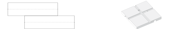
Overlap Joint - Overlap based on application - Angled or vertical surfaces - Used to direct water - Minimizes wind load pressure - Double color effect at joint
